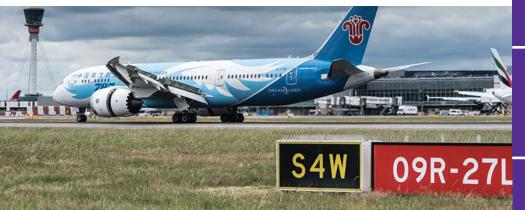
The example above indicates that you are at location S4W, holding short of Runway 09R/27L. The Runway 09R threshold is to your left; the Runway 27L threshold is to your right.
