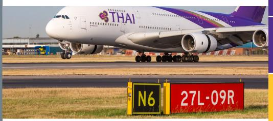
The example above indicates that your location is N6, holding short of Runway 27L/09R. The Runway 27L threshold is to your left, and the 09R threshold to your right.
