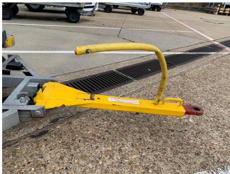
Damaged Baggage dolly safety barrier / safety hoop – dolly not to be used
