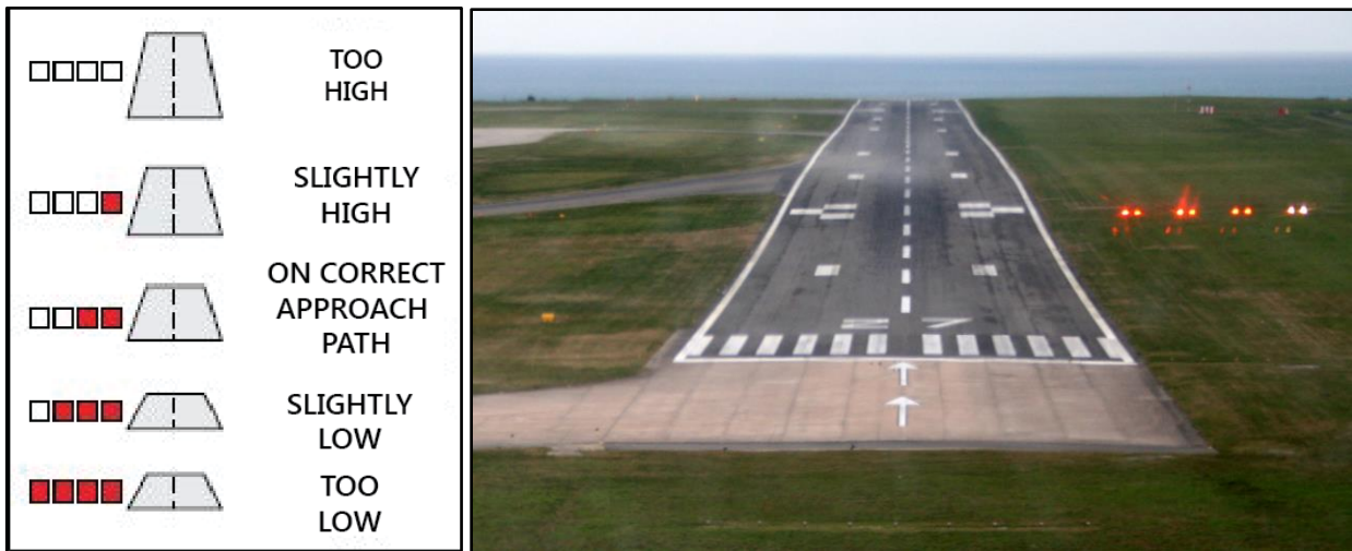
Figure 43: Precision Approach Path Indicators (PAPIs)
