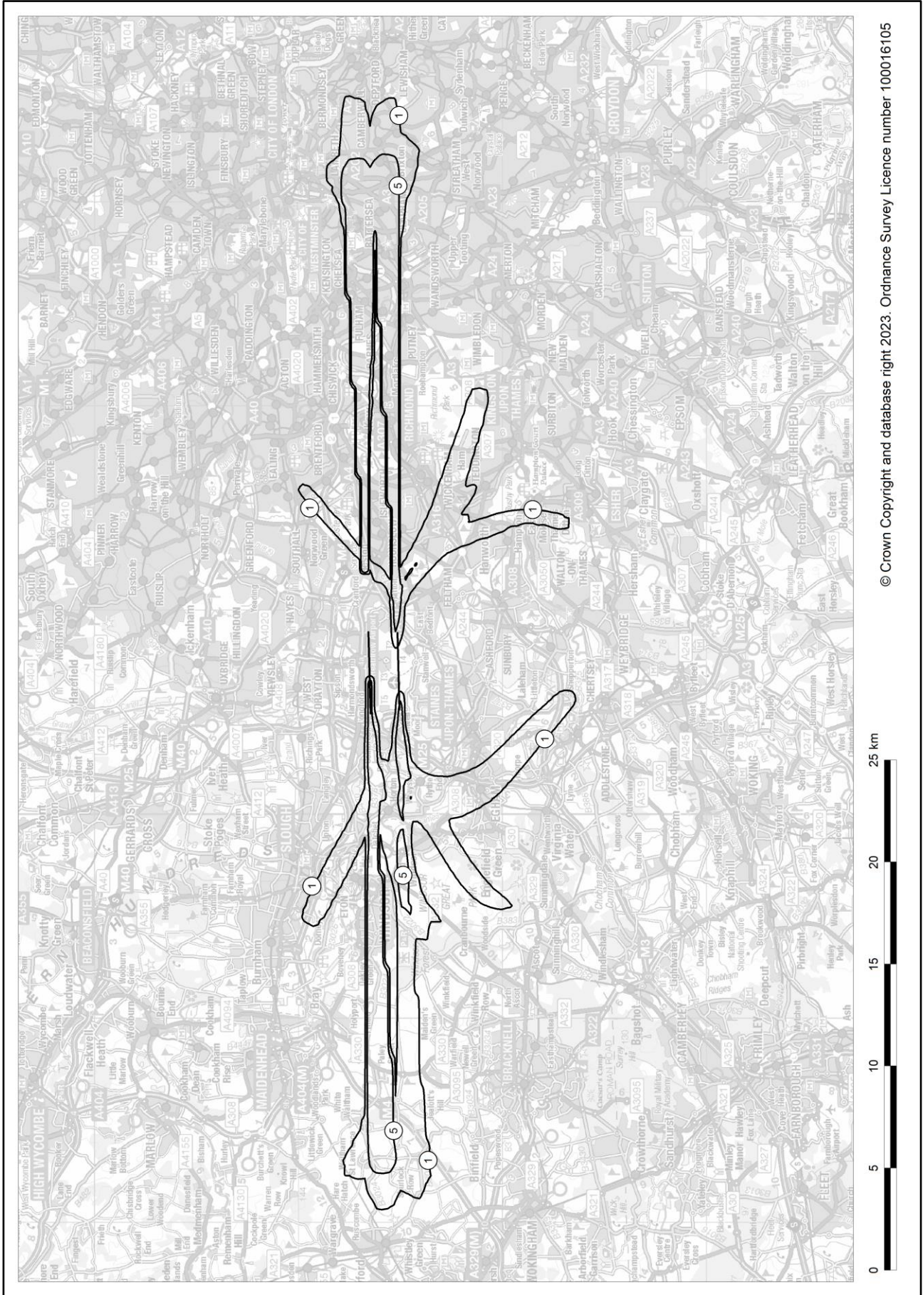
Figure B12b Heathrow 2022 average summer night overflight contours (assuming 60-degree elevation angle)
