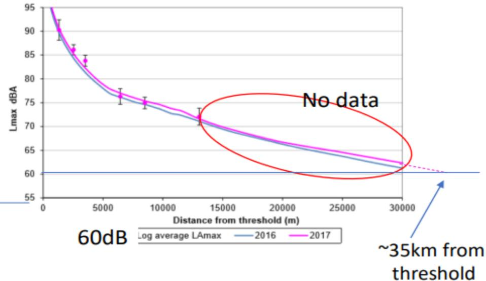
Figure E16 Airbus A320/CFM engines arrival  $L_{max}$
