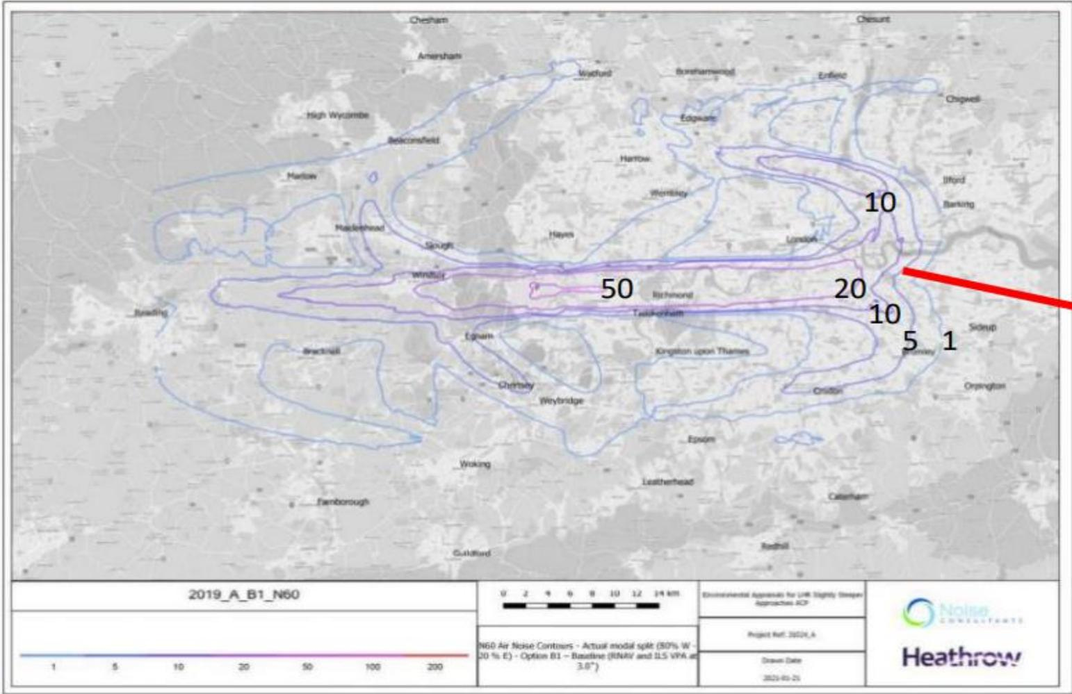
Noise Consultant modelling using latest flight dispersion, heights and and curved segments based on AEDT / INM modelling
